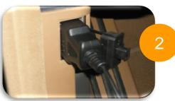
**Step #2** - Connect the power cable to the car's OBD11 connector
